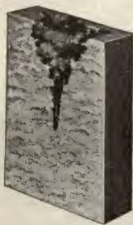
No. 1 Pipe Defect.
