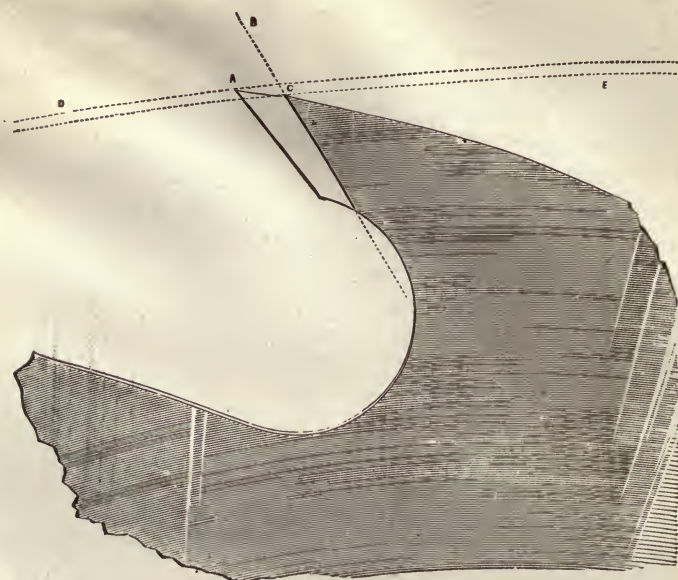
Illustration of Tooth after cutting 300,000 feet of Lumber.
